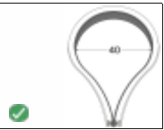
Fold the neon strip at top light emitting direction (as above photo). The minimum bending diameter is 40mm
