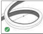
Circle Bending, top light emitting Face inside or outside. (A) Minimum diameter 50mm
