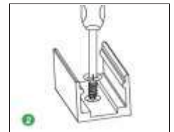
Fix the clip at appropriate area by screws
